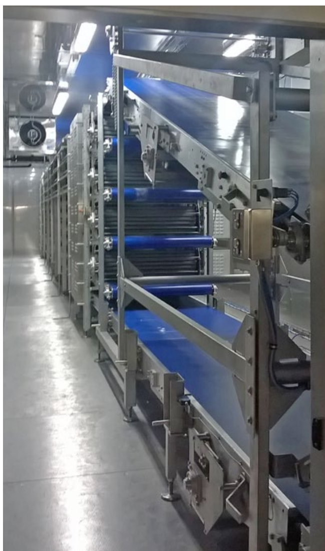
++ The cooling cell for the laminated doughs consists of several levels
