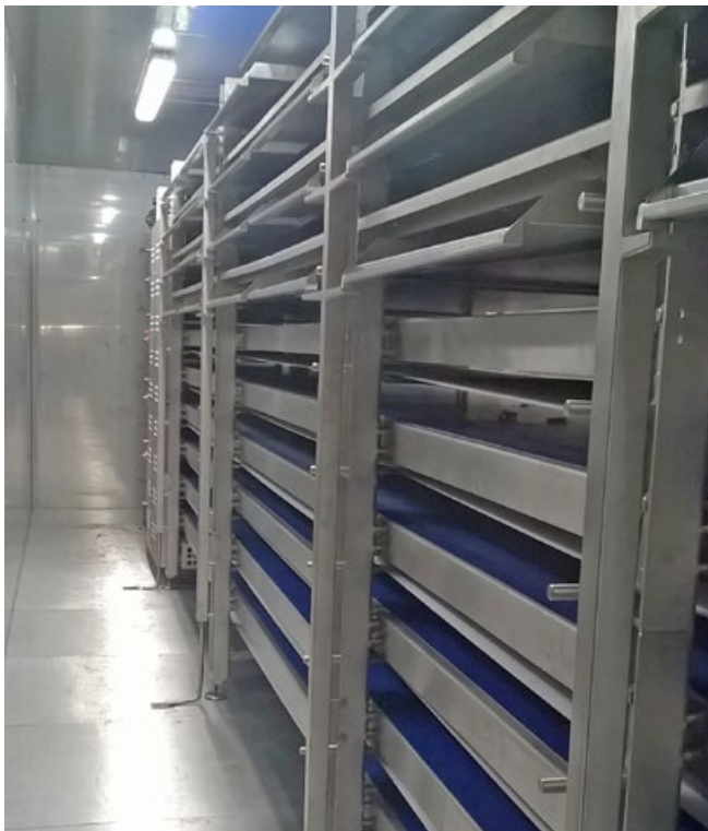
++ The stainless steel plates are modularly integrated into the cooling tunnel's conveyor belt system
