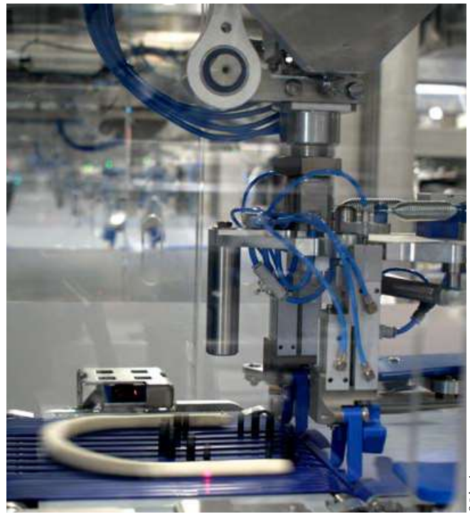
++ Looping the dough strands. Exchanging the tool also allows the production of other baked products, e.g. plaits or knots
