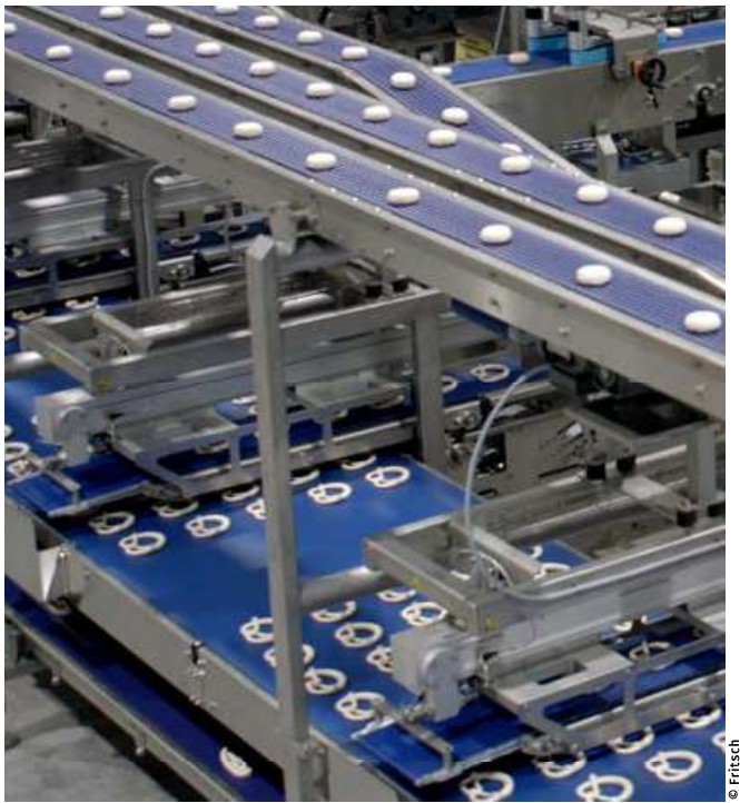
++ A total of ten looper modules enables an hourly output rate of 20,000 pretzels, bread rings, bread rolls or rolls
